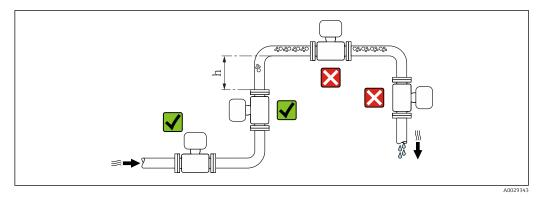
Preferably install the sensor in an ascending pipe, and ensure a sufficient distance to the next pipe elbow:  $h \ge 2 \times DN$
