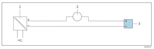
■ 14 Connection example for 4 to 20 mA current input
