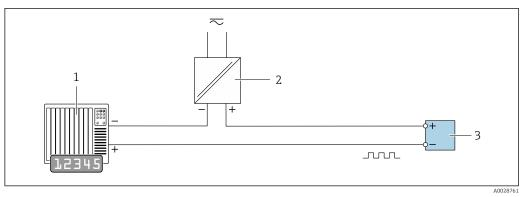
11 Connection example for pulse/frequency output (passive)
