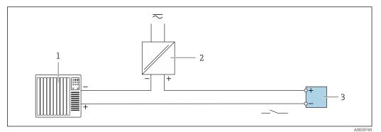
■ 13 Connection example for relay output (passive)
