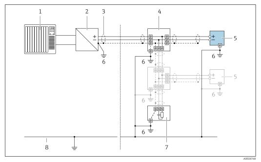
Connection example for FOUNDATION Fieldbus
