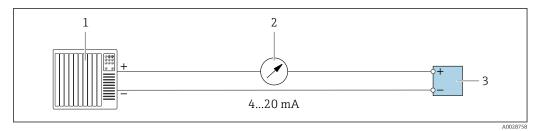
Connection example for 4-20 mA current output (active)
