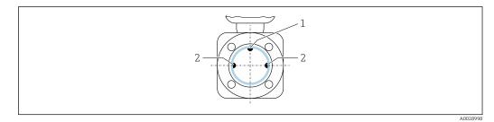
1 EPD electrode for empty pipe detection
