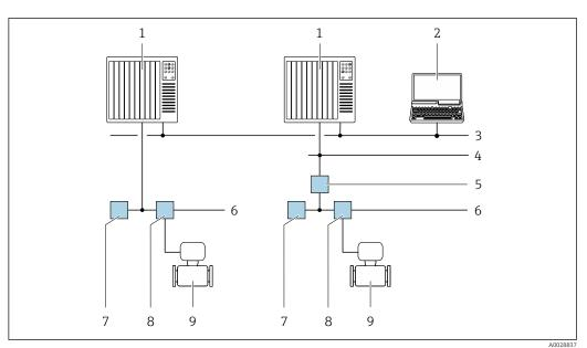
■ 18 Options for remote operation via FOUNDATION Fieldbus network
