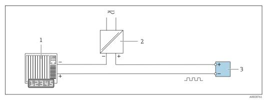
12 Connection example for pulse/frequency output (passive)
