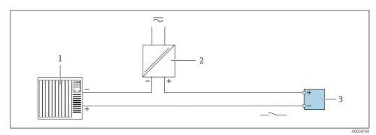
2 13 Connection example for switch output (passive)
