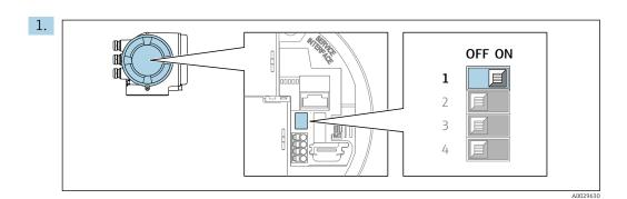
Setting the write protection (WP) switch on the main electronics module to the **ON** position enables hardware write protection.
