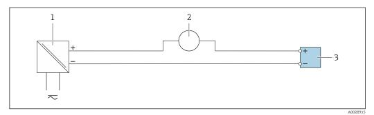
**■** 15 Connection example for 4 to 20 mA current input
