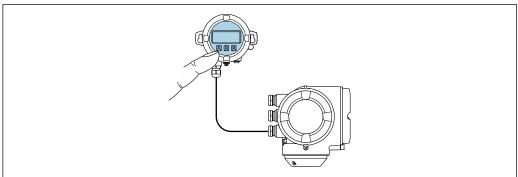
■ 31 Operation via remote display and operating module DKX001
