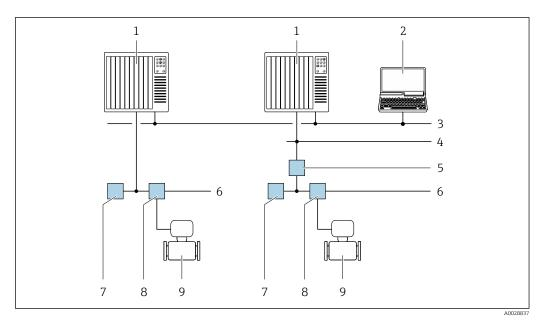
■ 19 Options for remote operation via FOUNDATION Fieldbus network
