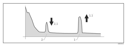
Vessel partly full, interference echo obtained
