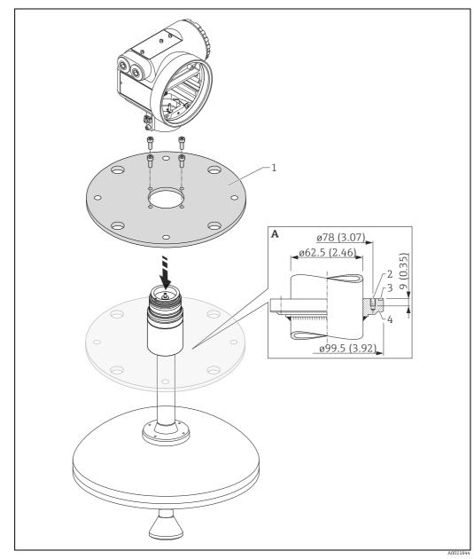
Α Flange hub for the connection to flanges provided by the customer. Dimensions: mm (in).
