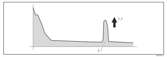
Vessel partly full, no interference echo obtained
