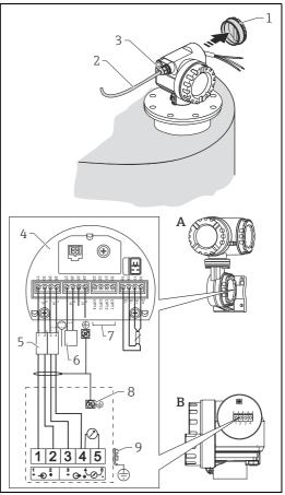
Tank Side Monitor NRF590 Micropilot S Housing cover Cabel Cable gland Intrinsically safe terminal board Only for Micropilot S HART Sensor Grounding single sided on Tank Side Monitor NRF590 Shielding cable DML (catential condication line)
