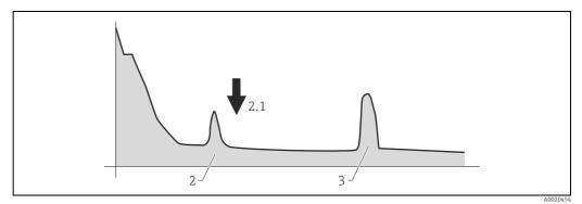
Vessel empty, interference echo obtained
