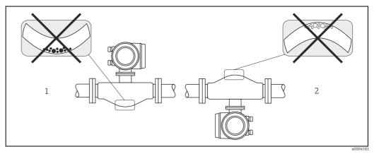
Horizontal installation for sensors with a bent measuring tube
