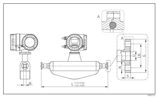
Detail A: The flange has the smaller groove for the O-ring on the sensor side. When mounting the sensor the corresponding flange must have accordingly a larger groove. Engineering unit mm (in).
