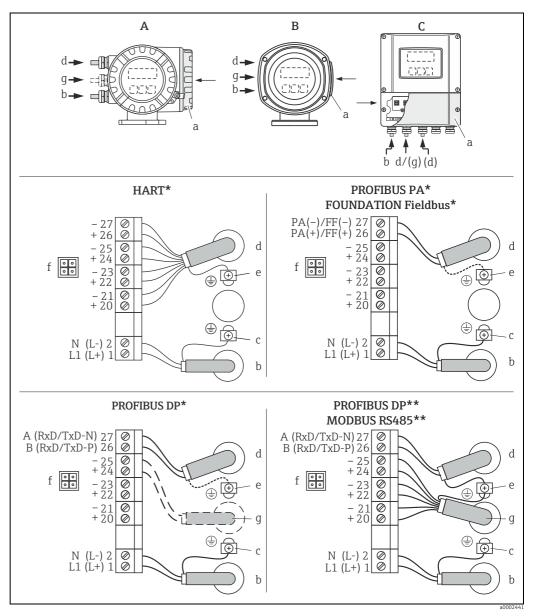
Connecting the transmitter, cable cross-section: max. 2.5 mm<sup>2</sup>
