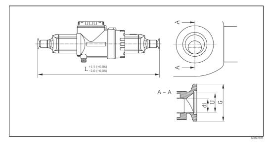
Neumo BioConnect clamp eccentric, DIN 11866 line A, clamp form R
