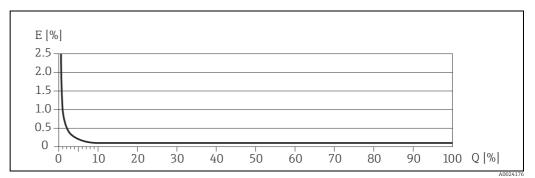
E = Error: Maximum measured error as % o.r. (example Promass 83P)
