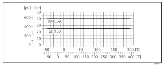
DIN 11851 allows for applications up to +140  $^{\circ}$ C (+284  $^{\circ}$ F) if suitable sealing materials are used. Please take this into account when selecting seals and counterparts as these components can limit the pressure and temperature range.
