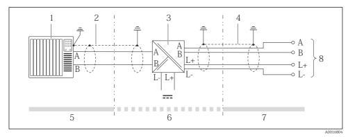
■ 11 Electrical connection between the transmitter and Safety Barrier Promass 100
