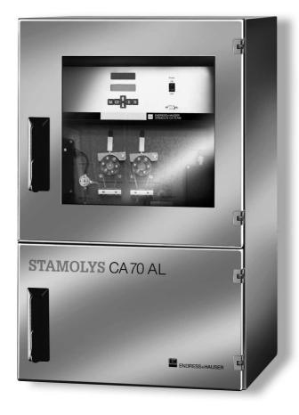
The StamoLys Analyzer CA 70 AL is a compact analysis system for low range concentrations of aluminum for use in drinking water and wastewater applications. Aluminum is determined using the photometric measuring principle.
