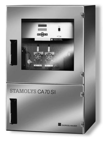
The StamoLys Analyzer CA 70 SI is a compact analysis system for silicate for use in ultrapure water and boiler feedwater. Silicate content is determined using the photometric measuring principle.
