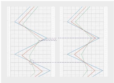
Left strip chart is without time offset compensation Right strip chart is with time offset compensation switched on
