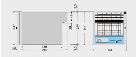
144x144x215mm panel mounted unit Panel cutout required 138<sup>+1</sup> x 138<sup>+1</sup> mm
