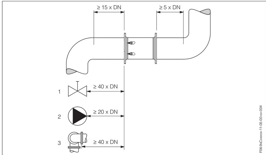
Fig. 9: Inlet and outlet runs
