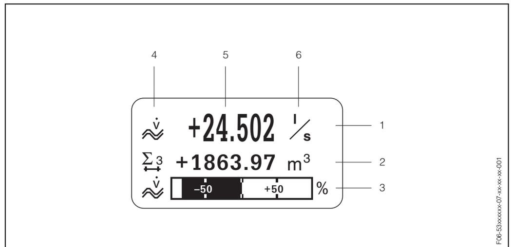
Fig. 25: Typical display for normal operating mode (HOME position)
