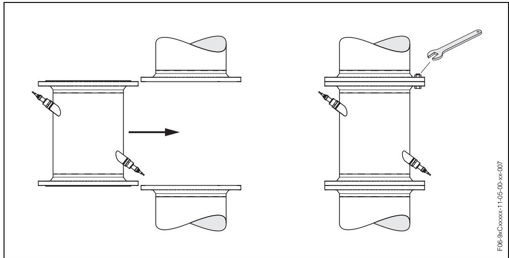
Fig. 13: Mounting measuring tube Prosonic Flow C
