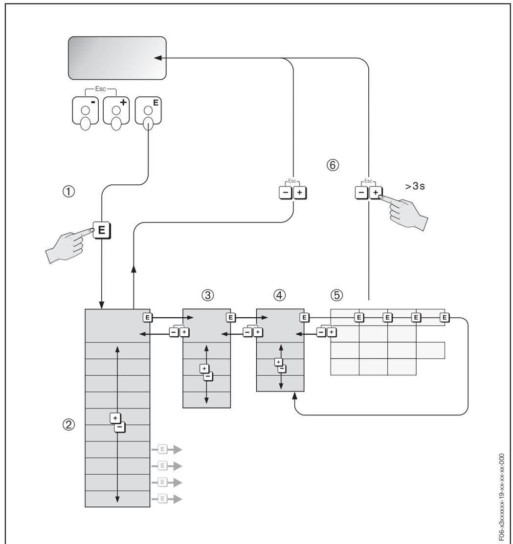
Fig. 26: Selecting functions and configuring parameters (function matrix)
