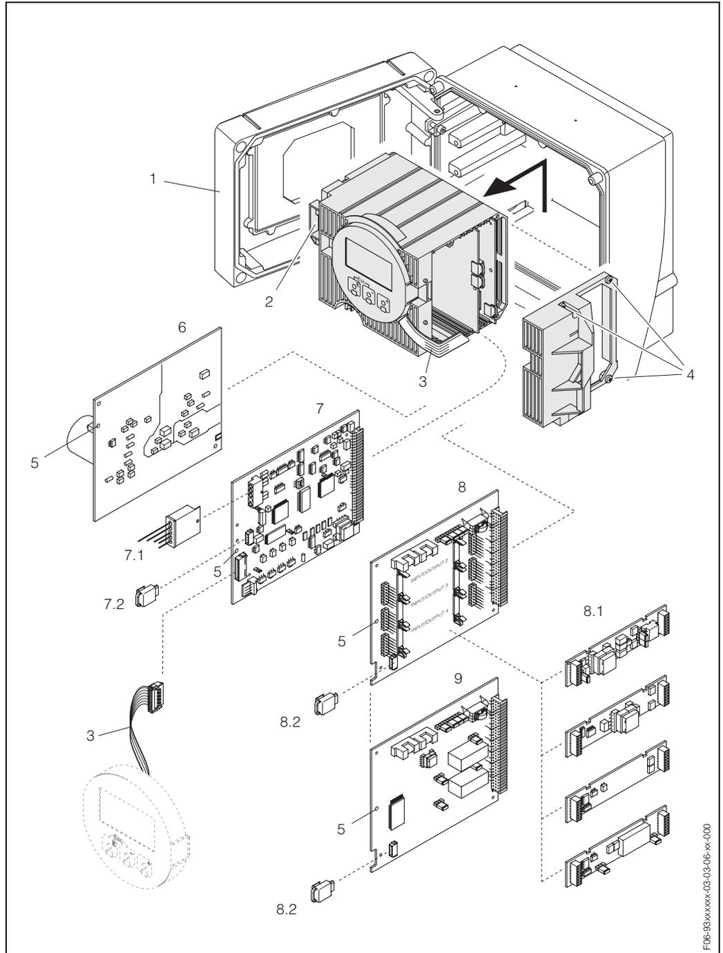
Fig. 37: Wall-mount housing: removing and installing electronics boards
