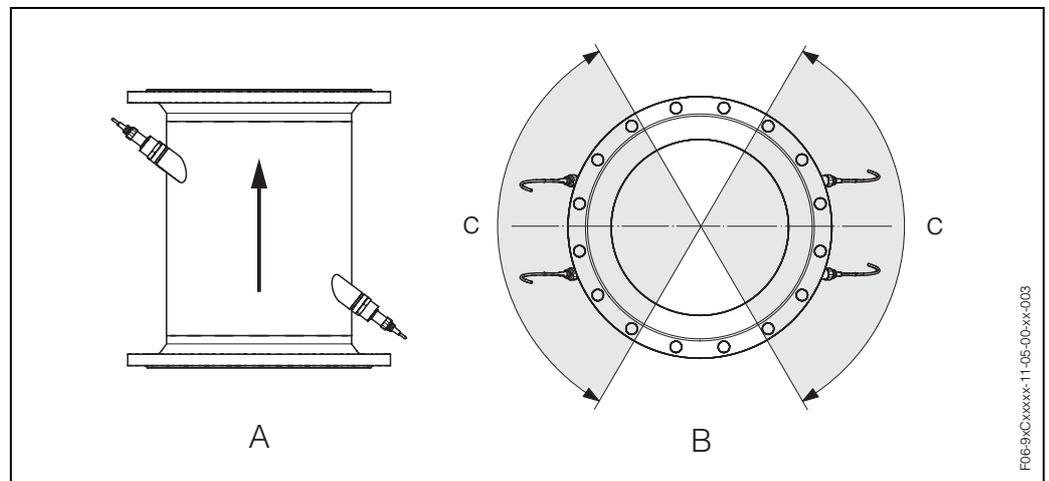
Fig. 8: Installation position (A = Vertical, B = Horizontal, C = Recommended installation range max. 120°)
