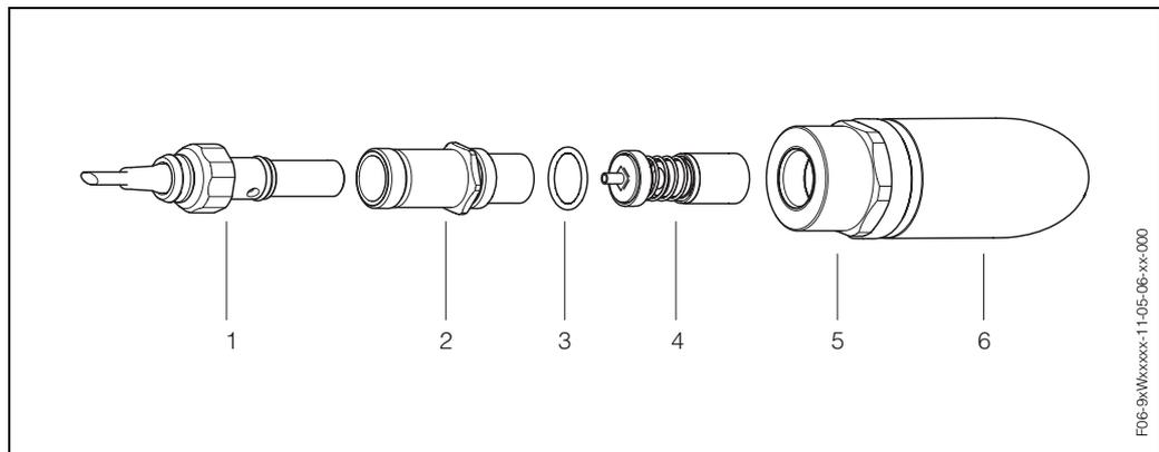
Fig. 38: Flowmeter sensor W: installation/removal
