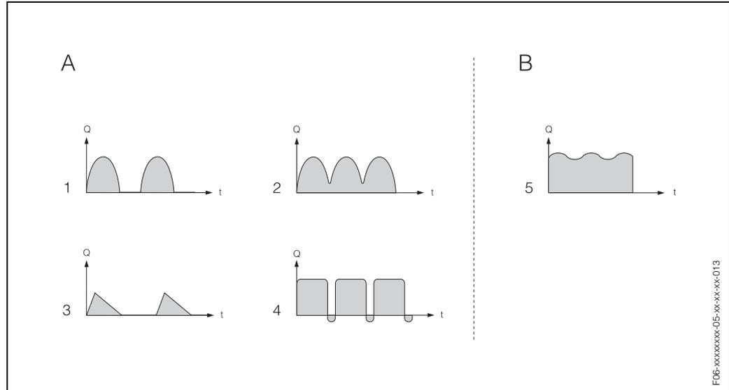
Fig. 30: Flow characteristics of various types of pump
