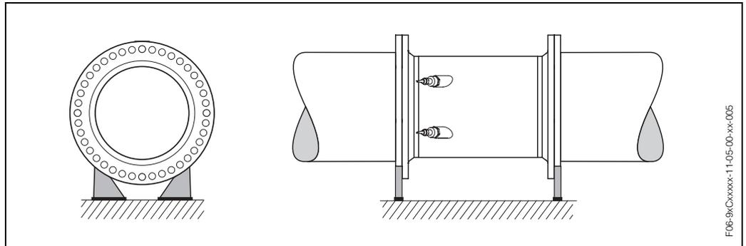
Fig. 11: Correct support for large nominal diameters
