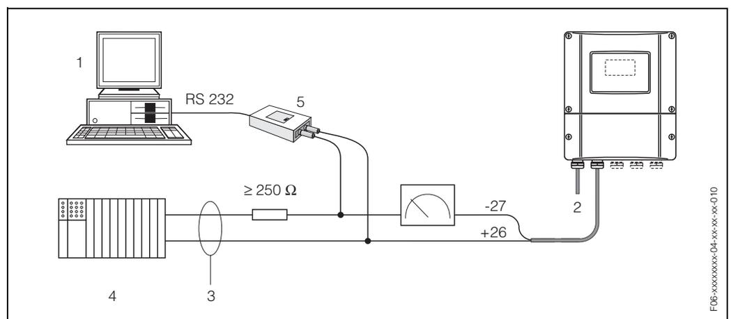
Fig. 21: Electrical connection of a PC with operating software
