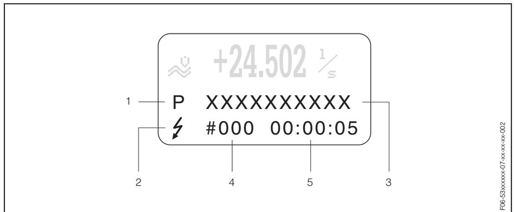
Fig. 27: Error messages on the display (example)
