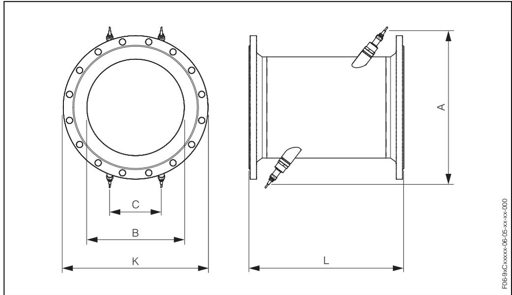
Fig. 42: Dimensions of measuring tube with installed sensors
