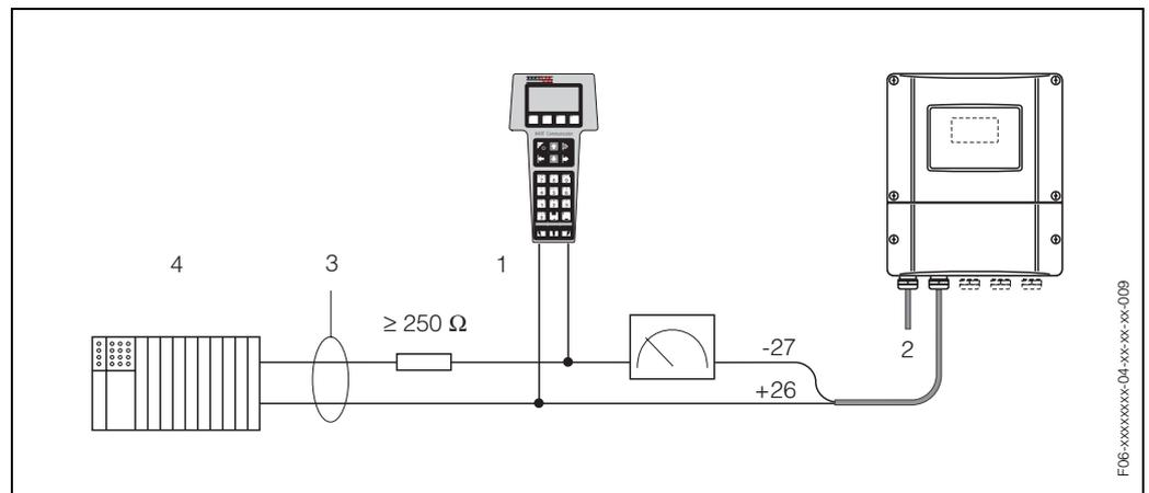
Fig. 20: Electrical connection of the HART handheld communicator:
