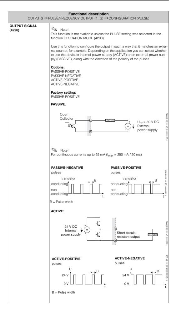
OUTPUTS → PULSE/FREQUENCY OUTPUT (1...2) → CONFIGURATION (PULSE)
