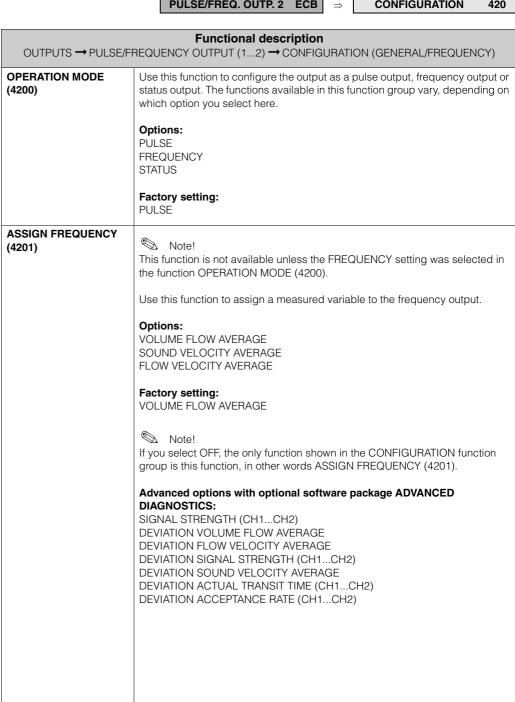
OUTPUTS → PULSE/FREQUENCY OUTPUT (1...2) → CONFIGURATION (GENERAL/FREQUENCY)
