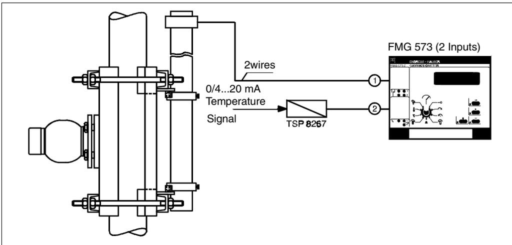
Fig. 5.2 Arrangement for temperature compensated density measurement with 4...20 mA Temperature signal and TSP 8267 converter
