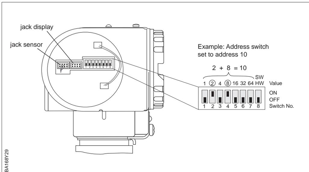
Figure 3.2 Cerabar S address switch
