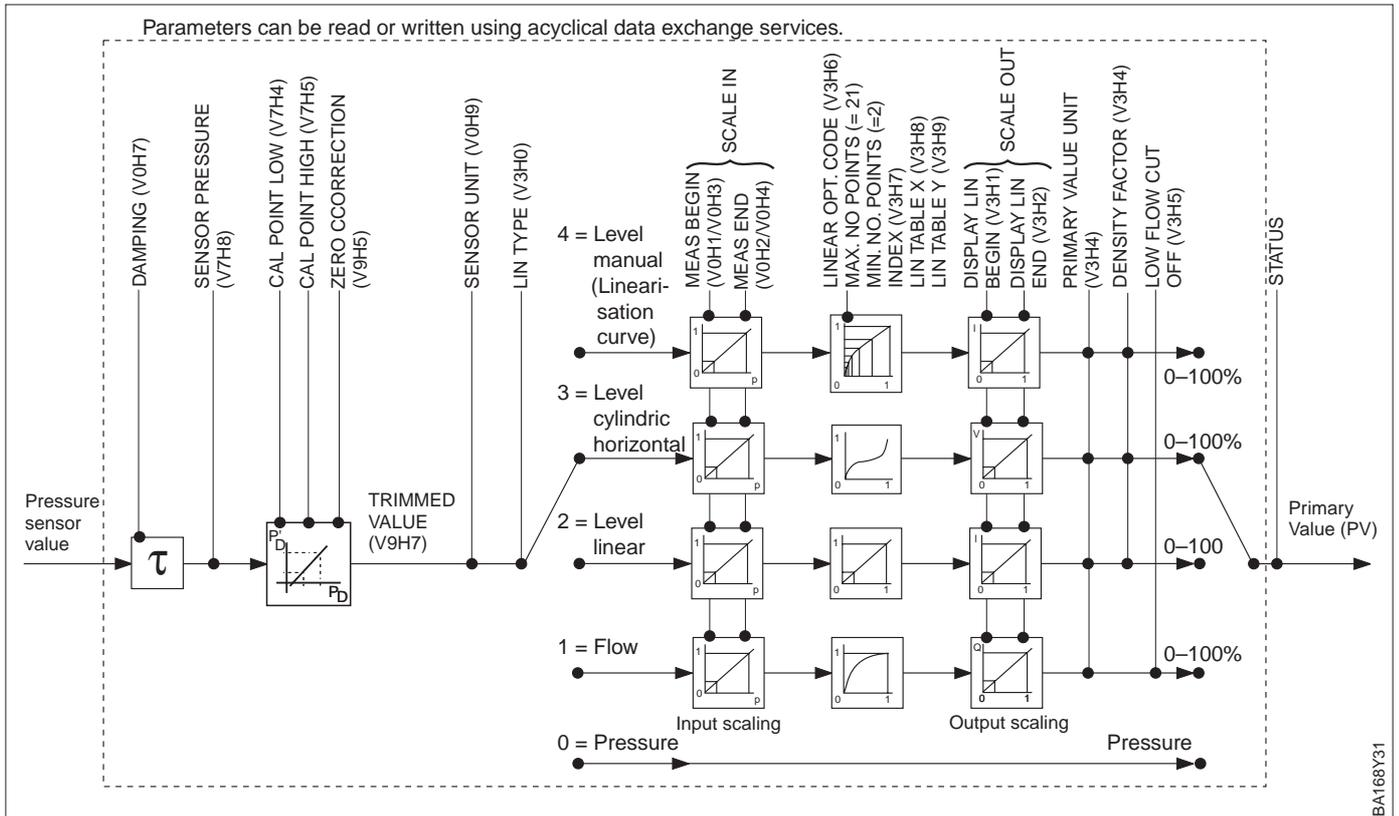
Figure 3.5 Schematic diagram of the Cerabar S transducer block. Parameter designations correspond to those designations in the Slot/Index List. Parameters with data for a matrix field (in brackets) can be accessed by Commwin II. The flow measurement is only relevant for differential pressure transmitters.
