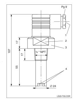
Dimensions CLS 20 with thread 1/2" NPT 1 Cable entry 2 36 AF 3 PES shaft
