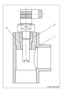
Installation of the measuring cell in a standard DN 32, 40 or 50 cross or T-piece by using a bonded adapter coupling. No adapter is required for installation in DN 25 crosses or tees.
