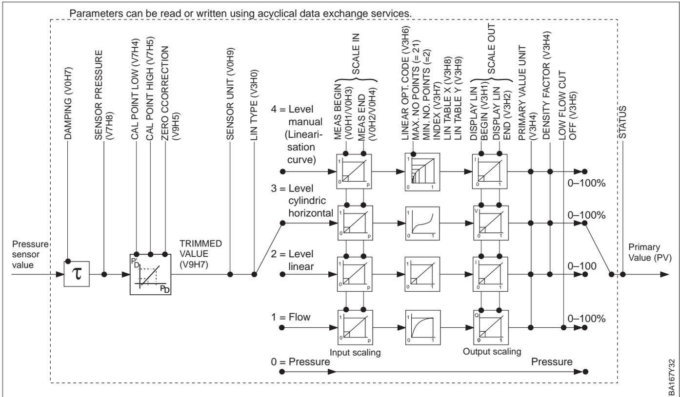
Figure 3.5 Schematic diagram of the Deltabar S transducer block. Parameter designations correspond to those designations in the Slot/Index List. Parameters with data for a matrix field (in brackets) can be accessed by Commuwin II.
