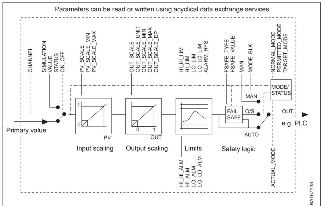
Figure 3.4 Schematic diagram of the Deltabar S analog input block
