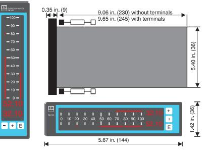
$\begin{array}{c} \mbox{Required panel cutout} \\ (\mbox{to DIN 43700}) \\ 54.4 \mbox{ in. x 1.3 in.} \\ (\mbox{138}^{+1} \mbox{ mm x 33}^{+0.6} \mbox{ mm}) \end{array}$
