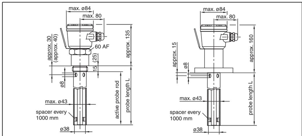
left: Multicap DC 11 with threaded boss G 1 1/2 A and **ground tube**
