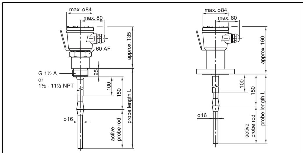
left: Multicap DC 11 with threaded boss and **active build-up compensation**
