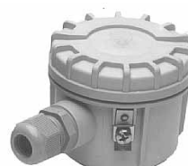
Order code K Polyester (PBTP) housing IP66 with cable gland PG 16
