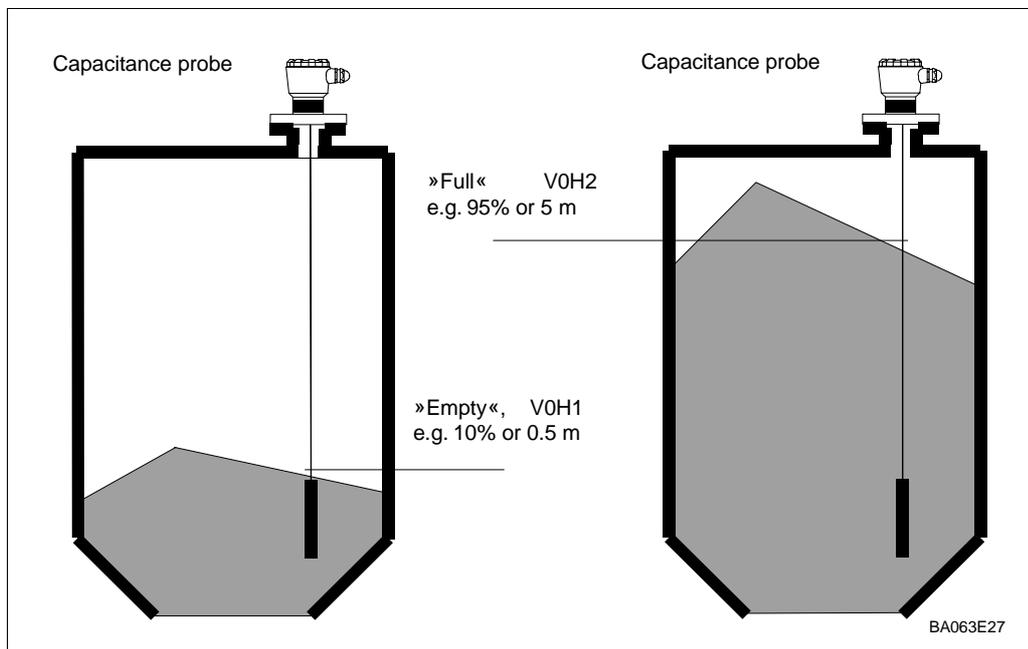
Fig. 4.1: Parameters required for calibration of the Silometer FMC 671 Z/676 Z for level measurement shown for bulk solid measurement. Any filling mound or outflow depression can be accounted for by the parameters entered.
