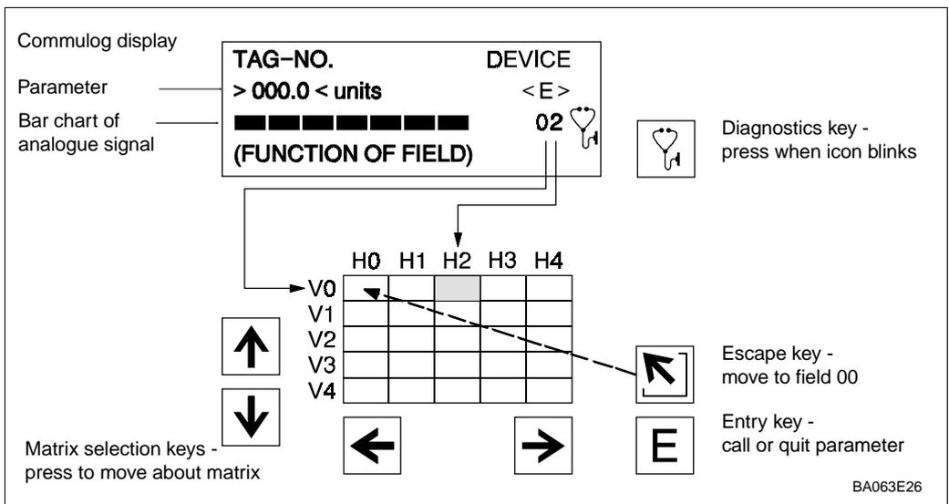
Fig. 3.2: Commulog display and key functions for the Silometer FMC 671 Z/676 Z
