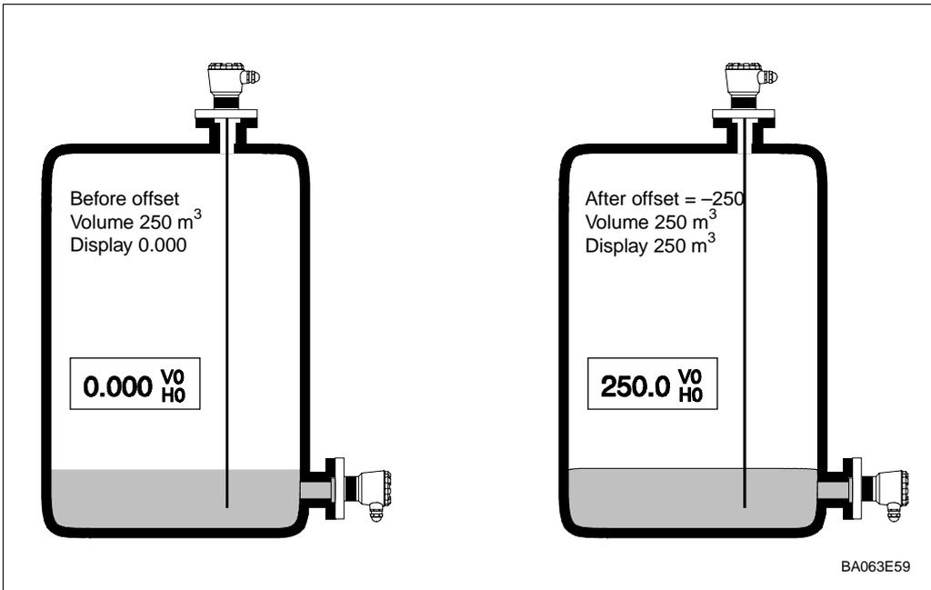
Fig. 4.3: Effect of level offset value on display at V0H0 for level measurement
