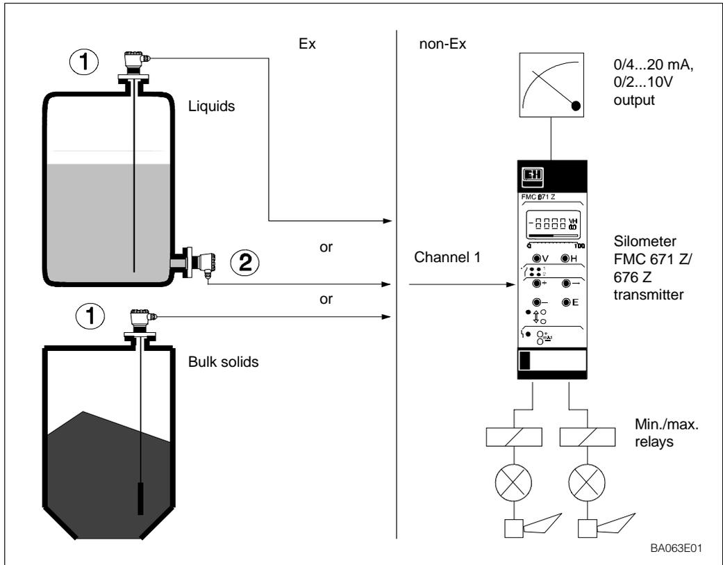
The Silometer FMC 671 Z/676 Z is designed for level measurement with a capacitance, impedance or hydrostatic pressure probe. A second channel allows level limit detection with a capacitance/impedance probe or vibration sensor. The applications described in this manual are as follows:
