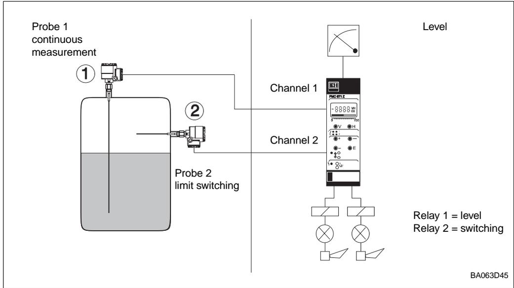
Operating mode 0 allows level measurement on channel 1 and level switching on channel 2. If a Deltapilot S is being used, only a Liquiphant can be used as limit switch. Each channel is assigned to a relay.
