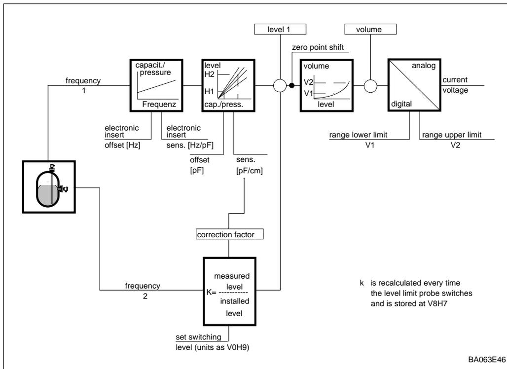
Fig. 8.6: Schematic diagram of automatic calibration correction
