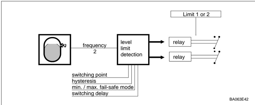
Fig. 8.2: Schematic diagram, limit level switching. Relay 1 must be assigned to channel 2 at V1H4
