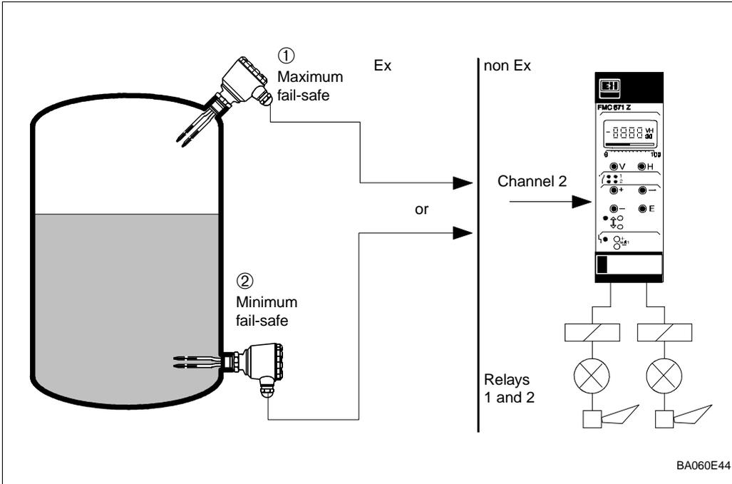
Fig. 8.4: Standard installation for limit switching with vibration sensors
