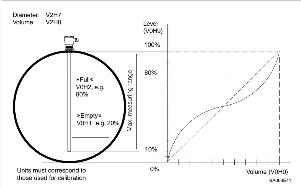
The Silometer FMC 671 Z/676 Z transmitter uses a stored linearization table which requires the entry of the tank diameter, tank volume for its volume calculations.
