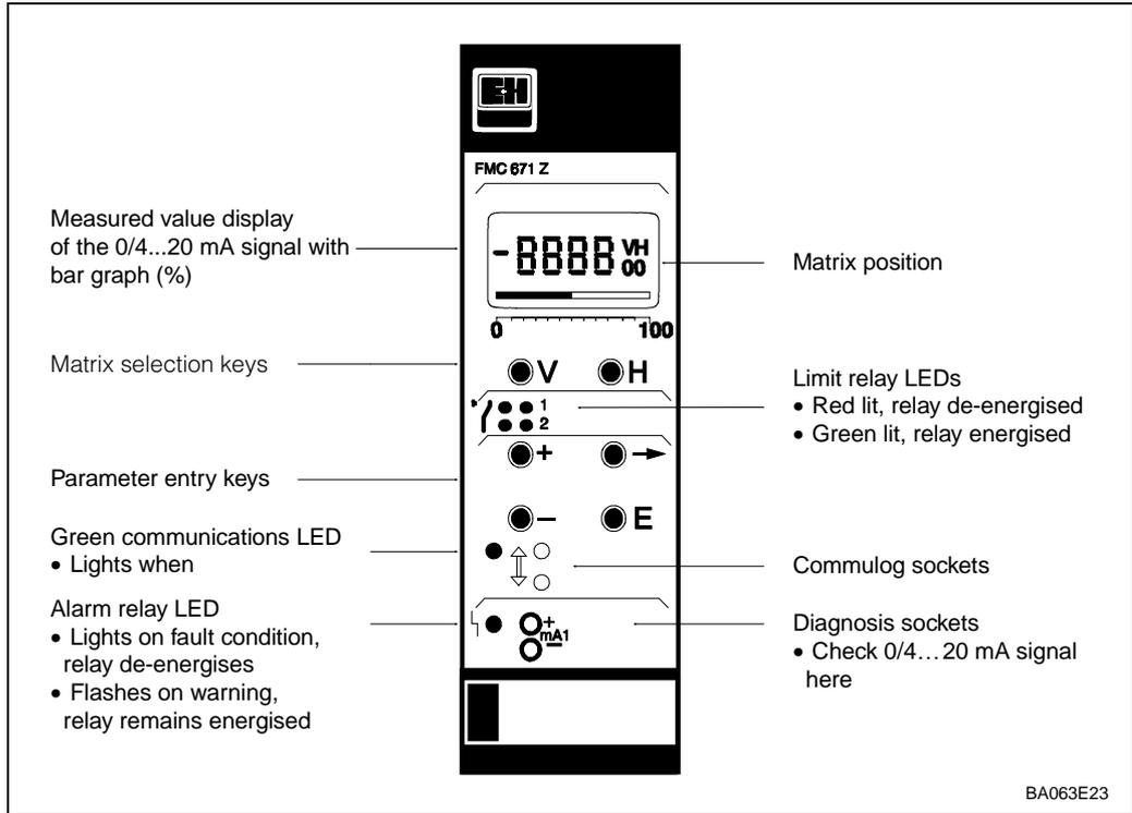
Fig. 3.1 shows the LC-display with matrix of the Silometer FMC 671 Z, Fig. 3.3 its front panel. Table 3.1 below describes the function of the operating keys.
