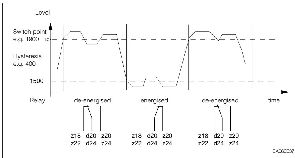
Fig. 7.2: Range switching with maximum fail-safe mode
