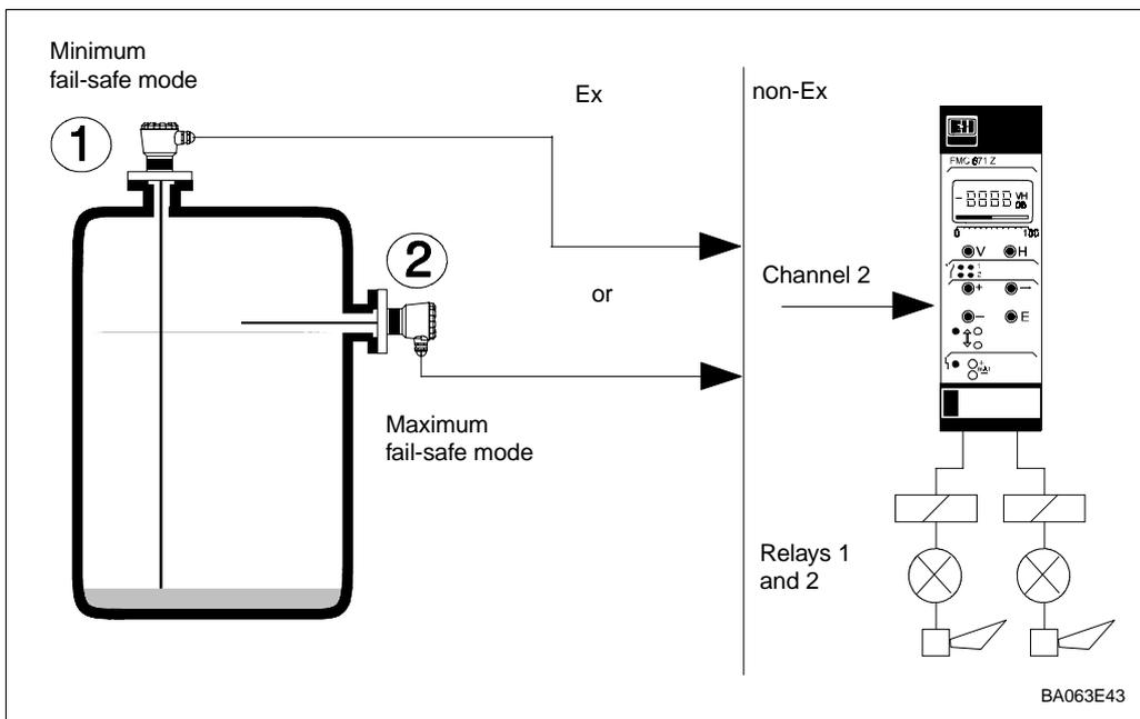
Fig. 8.3: Schematic diagram, limit level switching with capacitance probes. ① Minimum fail-safe, ② Maximum fail-safe
