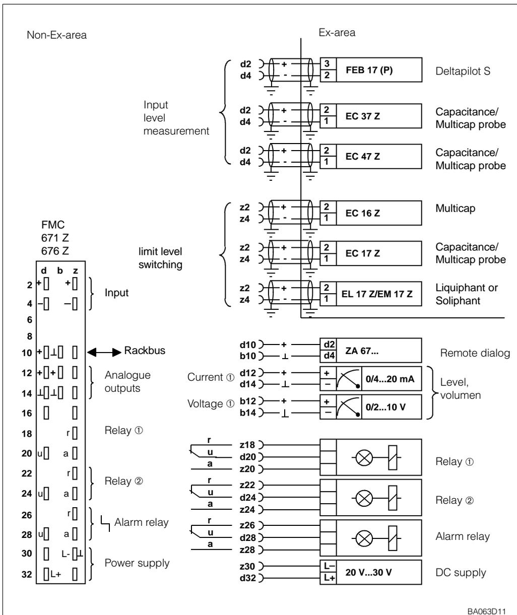
Fig. 2.4: Pin assignment diagram for Silometer FMC 671 Z/676 Z
