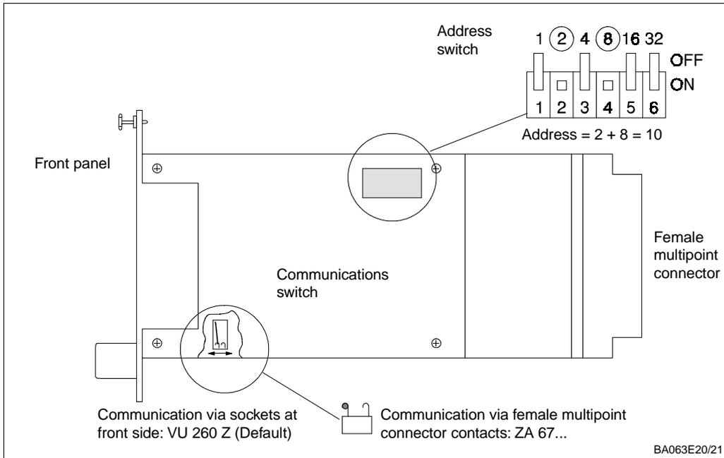
Fig. 2.10: Configuration elements of Silometer FMC 671 Z/676 Z shown for Commulog operation
