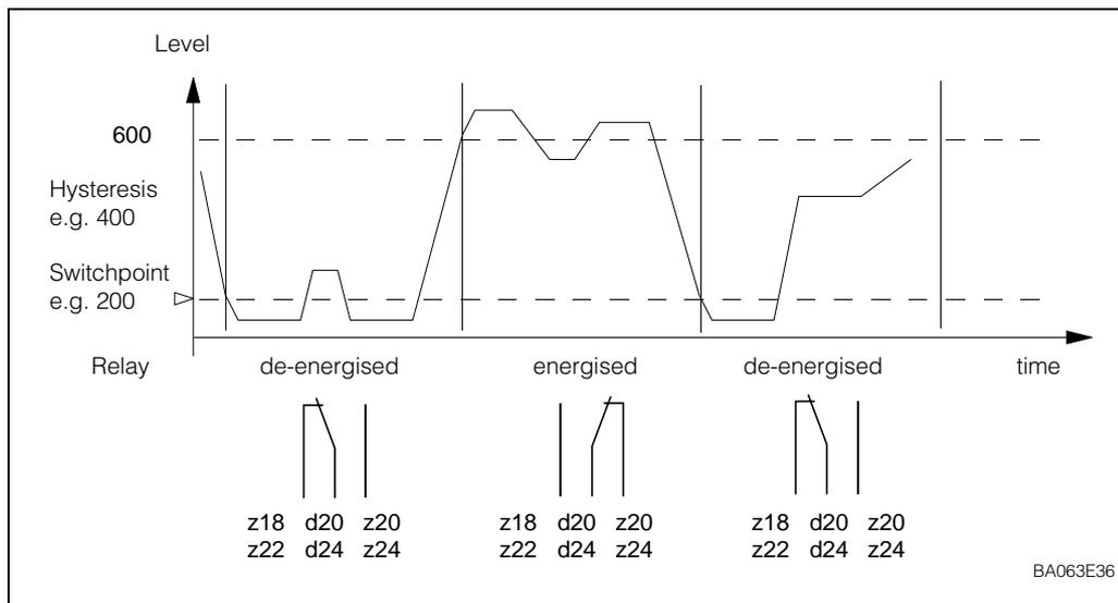
Fig. 7.1: Range switching with minimum fail-safe mode
