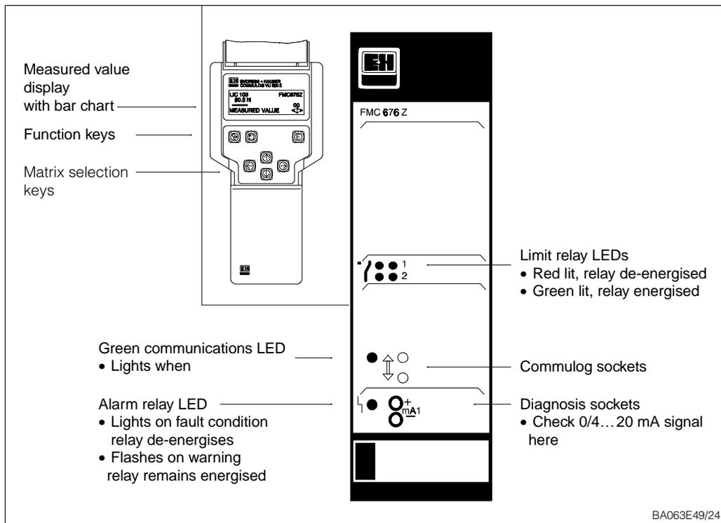
Fig. 3.4: Silometer FMC 676 Z Showing front panel and Commulog VU 260 Z key functions
