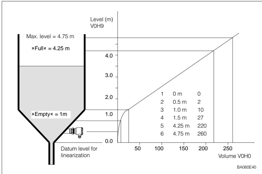
Fig. 5.3: Linearisation for a vessel with a conical outlet
