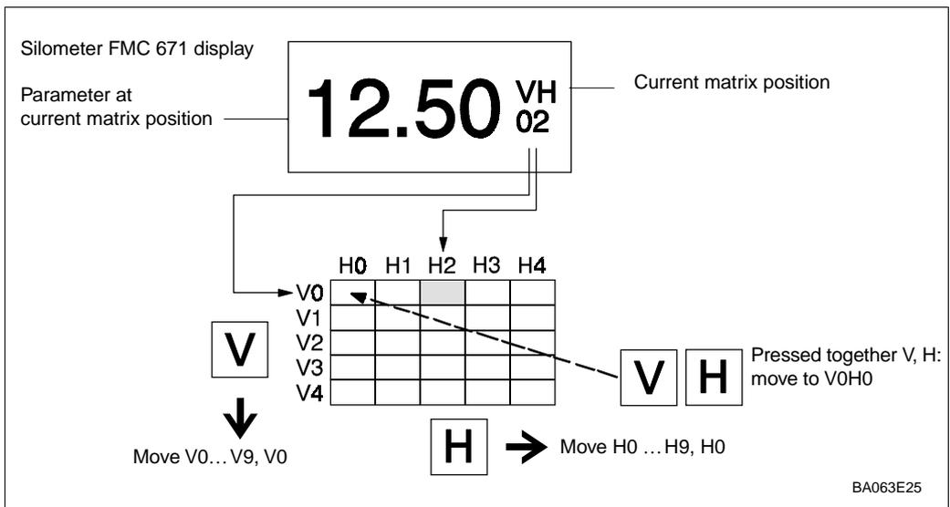
Fig. 3.1: Silometer FMC 671 Z Parameter matrix operation with function of V and H keys. The complete matrix has 10 x 10 fields, although not all are used
