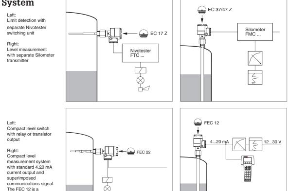
The FEC 12 is a "Smart electronic insert" which allows remote calibration over two-wire cabling (HART protocol)
