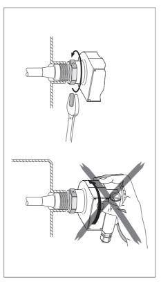
Probe with thread 1½ - 11½: Tighten ar the hexagonal nut
