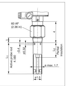
Left: DC 11 AN, fully insulated rod probe with ground tube
