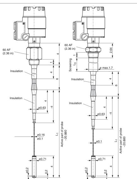
Left: rod probe DC 11 AS (fully insulated) or DC 16 AS (partially insulated)
