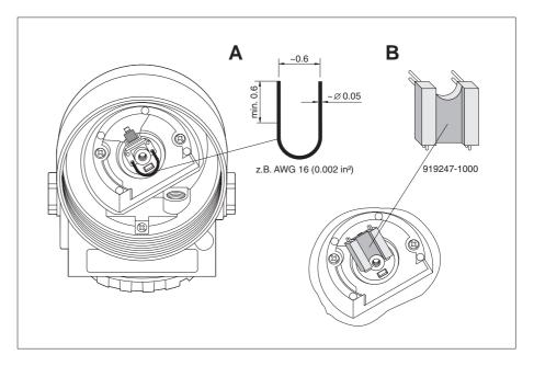
Grounding the probe rod or rope in the housing: A Jumper, e.g. made of uninsulated wire, AWG 16 (0.002 in<sup>2</sup>)
