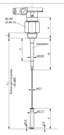
Left: DC 21 AN, fully insulated rope probe
