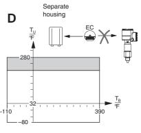
Mounting of the electronic insert as a function of operating temperature  $T_B$  and ambient temperature  $T_U$ :
