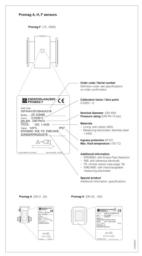
Fig. 2 Promag A, F, H sensors Typical nameplate specifications (example)
