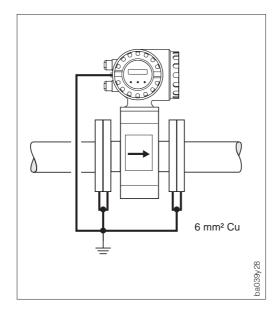
The fluid may be earthed. In order to make the most of the electromagnetic compatibility (EMC) of the Promag 30, it is advisable to provide two flange-to-flange links and to connect them jointly with the transmitter housing to earth potential.
