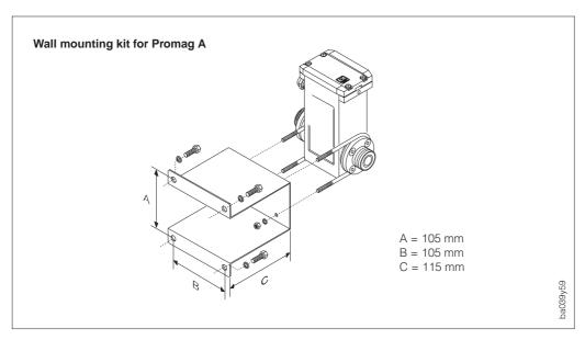
Fig. 38 Dimensions Wall mounting kit for Promag A
