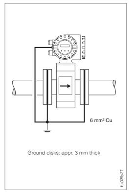
Ground disks must always be used with non-conductive piping materials if compensation currents flow through the fluid. They can irreparably damage the reference electrode within a short time due to electrochemical corrosion.
