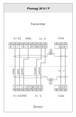
Fig. 26 Wiring diagrams for the remote versions "FS" and "FL"
