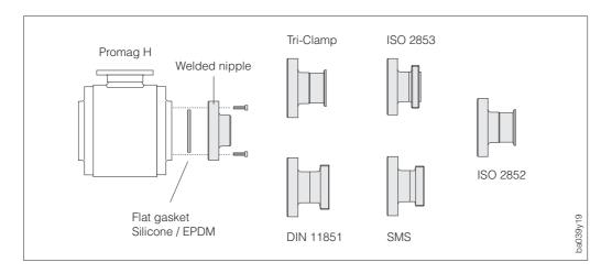
Fig. 14 Process connections Promag H
