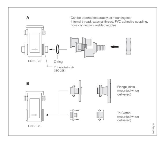
Fig. 13 Process connections Promag A
