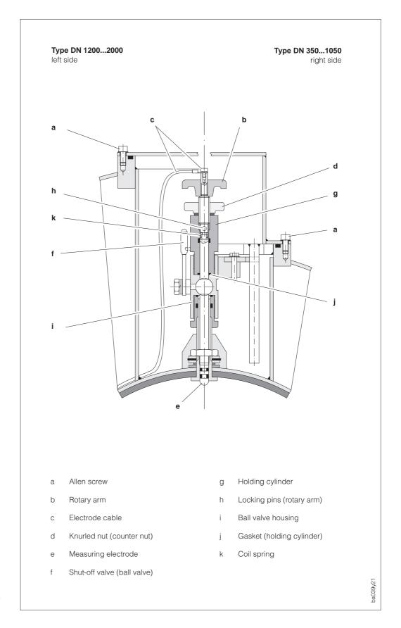
Fig. 35 Replacement unit for changing electrodes
