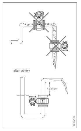
Correct measurement is only possible when the pipe is full. The following locations should therefore be avoided:
