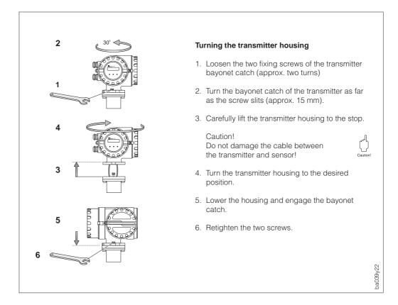
Fig. 16 Turning the transmitter housing
