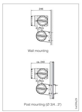
Fig. 18 Wall and post mounting
