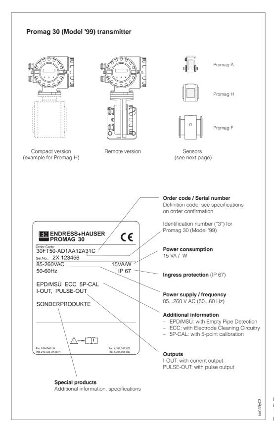
Fig. 1 Promag 30 transmitter. Typical nameplate specifications (example)
