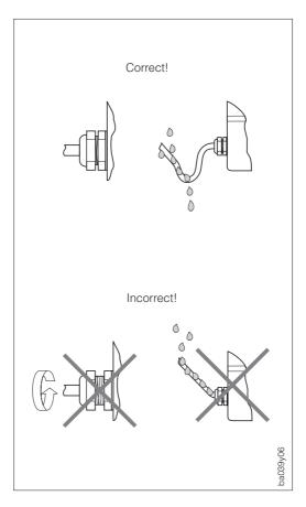
Fig. 20 Mounting cable entries
