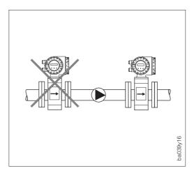
Fig. 8 Installation of pumps
