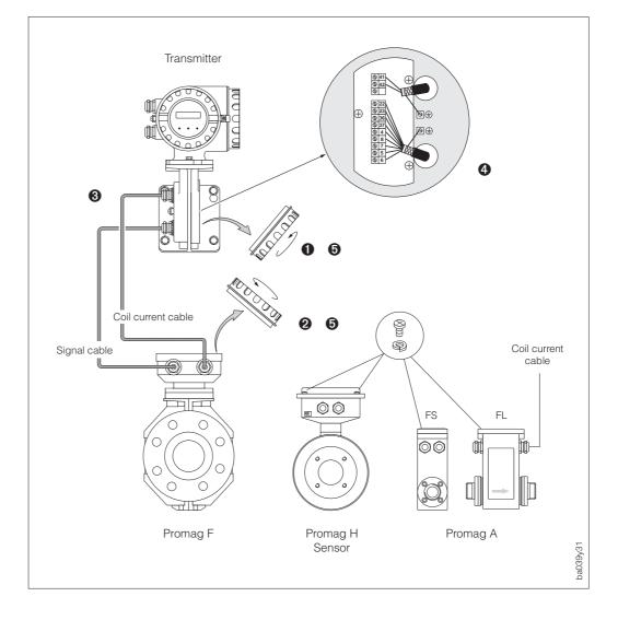
Fig. 25 Connecting the transmitter / sensor cable
