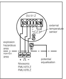
Intrinsically safe connection of the DU 51 Z ultrasonic sensor to the Nivosonic FMU 673 Z or FMU 678 Z using normal, unscreened, three-core multipurpose cable, max. 25  $\Omega$  per core.
