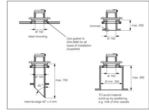
Mounting examples for closed tanks or silos
