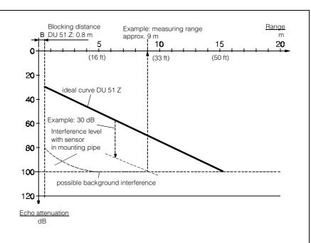
Example for calculating the range: (liquid tank):
