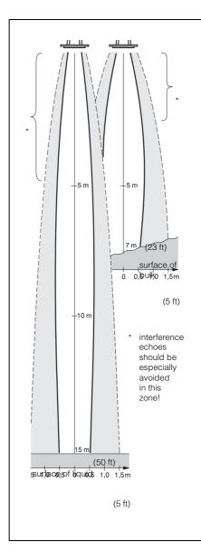
Detection zone as a function of application conditions. Continuous lines: good reflection characteristics, low attenuation giving low amplification in the Nivosonic FMU transmitter.
