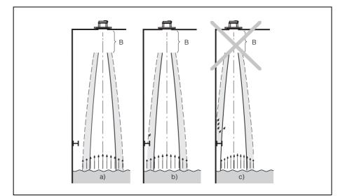
Avoid interference echoes from internal fittings and rough silo walls!
