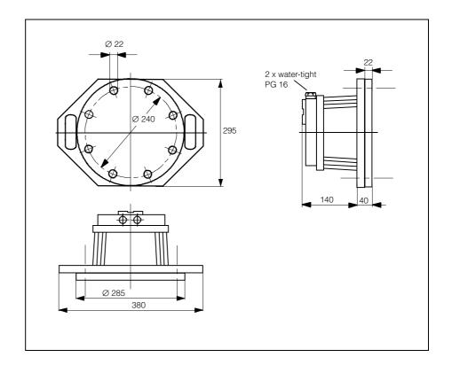
Dimensions of the DU 51 Z ultrasonic sensor in mm
