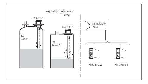
The ultrasonic measuring system for continuous, non-contact level measurement in tanks and silos
