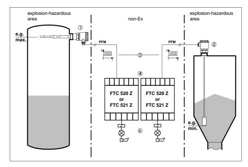
Measuring system for capacitance limit detection in liquids tanks and bulk solids silos
