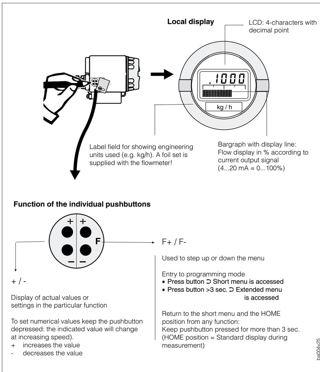
Fig. 41: Display and operating elements
