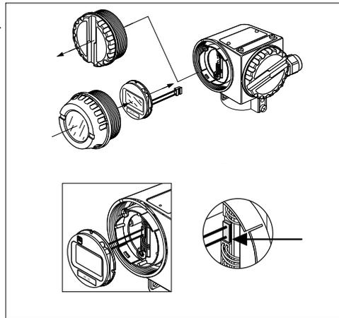
Fig. 29: Mounting/removing the local display module
