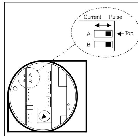
Fig. 31: Location of the pulse/current selection switches after removing the display and display bezel - remote electronic sensor version only
