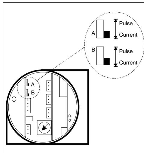
Fig. 30: Location of the pulse/current selection switches after removing the display and display bezel - compact sensor version only
