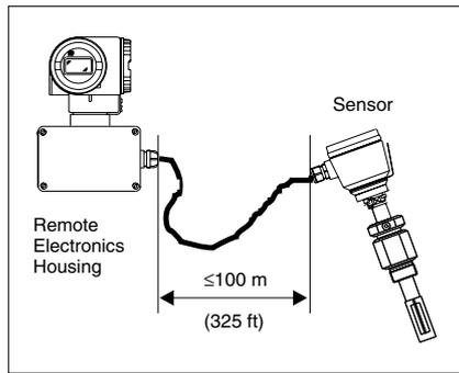
The AT70 sensor family can be supplied with the main electronics, display and keyboard contained in a remote housing that can be mounted up to 100m (325 ft) away from the sensor.
