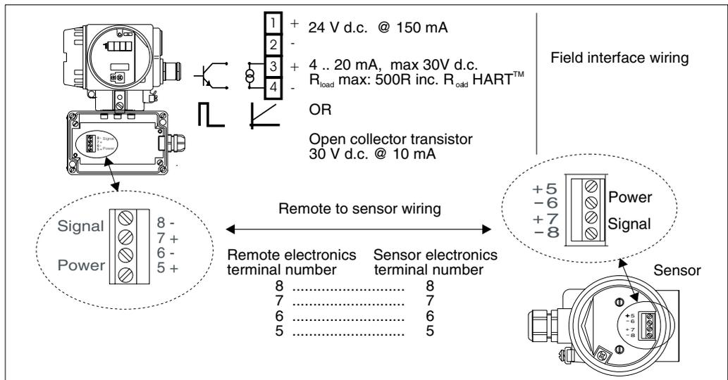
Fig. 37: General wiring schematic - Separated electronics housing and sensor
