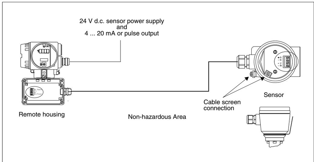
Fig. 38: Remote housing to sensor wiring - non-hazardous area operation
