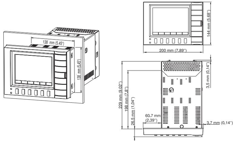
Dimensions for panel mounting on IP65 stainless steel version and rear panel or terminal cover, rear mounted ATA flash card drive
