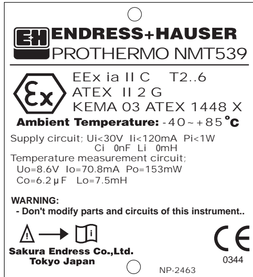
Fig 1 Information on the nameplate of the Prothermo NMT 539 with ATEX approval, "Converter only" version.
