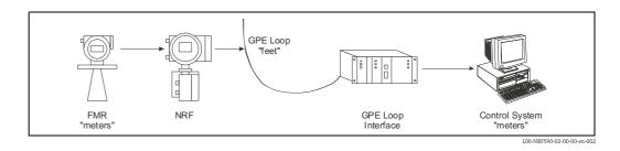
In this example, the NRF will have to be set to "feet" as the GPE loop is working in "feet". The NRF will convert the level from the FMR using the correct conversion factor (1ft = 0.3048m), however the GPE Loop Interface to the Control System may use an inaccurate conversion (e.g. 1ft = 0.3m). To compensate for this inaccuracy, the "Conversion Factor Adjustment" (CFA) value can be set as follows:
