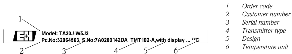
fig. 1: Nameplate of the TA20J (example with transmitter and display)
