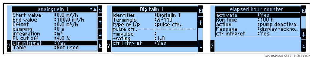
Fig. 24: Signal evaluation for analog inputs, digital inputs and elapsed hours counters
