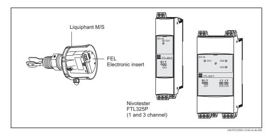
The safety-related signal of the measuring system is the level relay of the Nivotester. All safety functions refer
