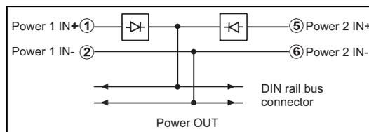
Block diagram power terminal block
