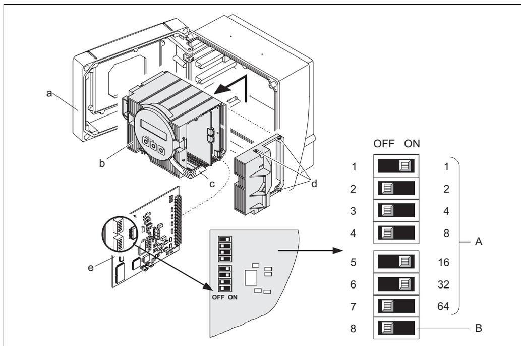
Fig. 47: Addressing using the miniature switches on the I/O board
