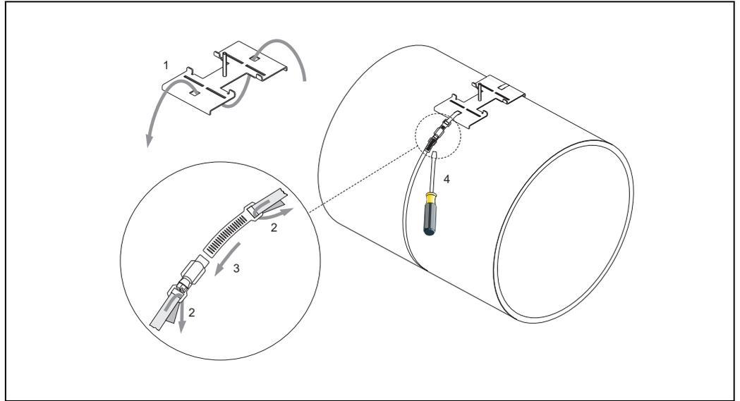
Fig. 12: Tensioning band installation for DN 250...4000
