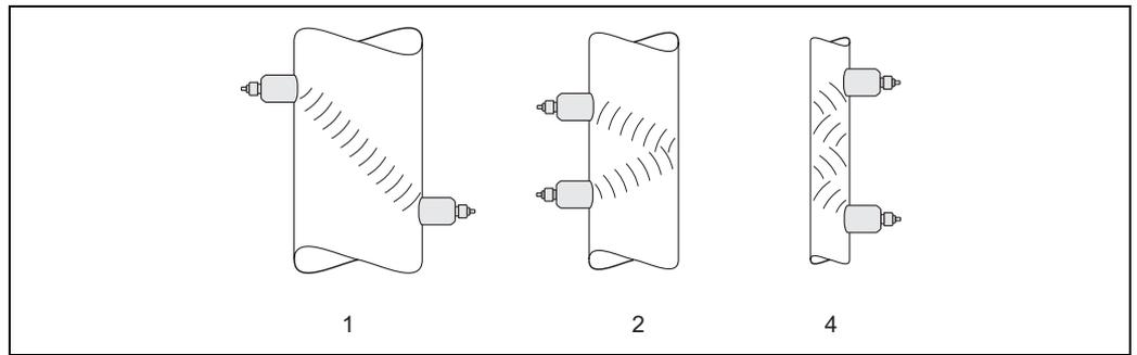
Fig. 10: Sensor arrangement (clamp-on)
