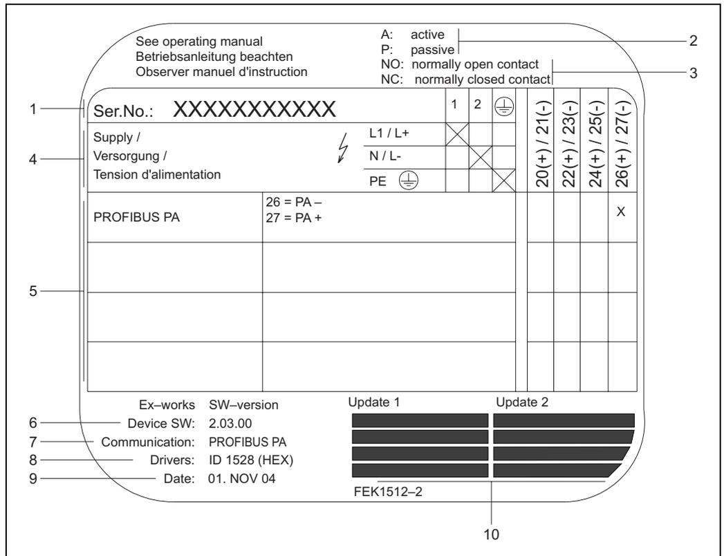
Fig. 4: Nameplate specifications for Proline transmitter (example)
