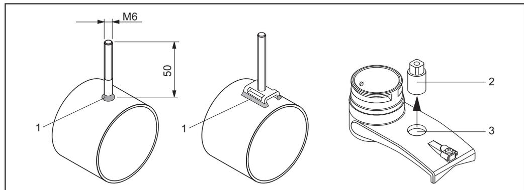
Fig. 13: Use of welded bolts
