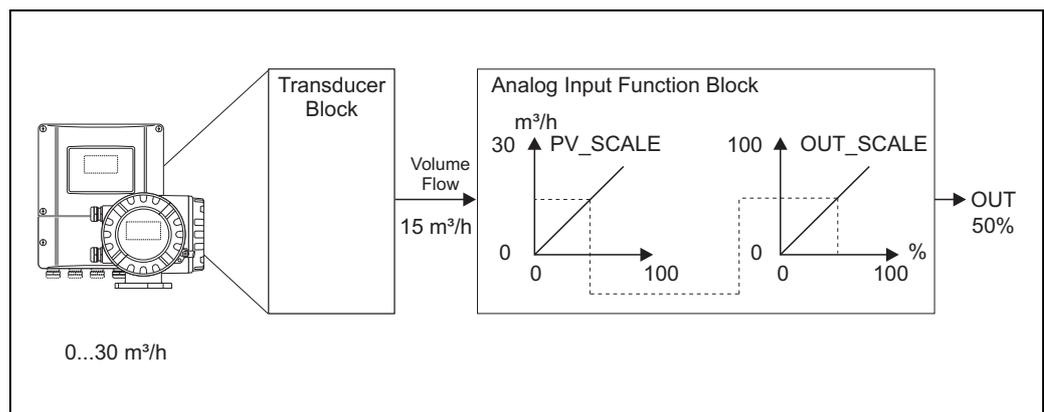
Fig. 50: Scaling the input value for the Analog Input function block
