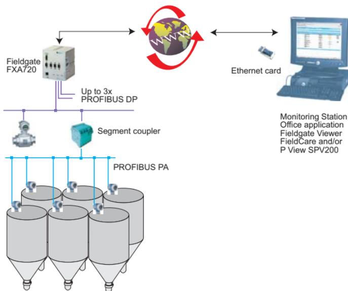
Example for installation in a control network:
