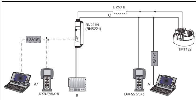
A = Connection HART® communication at 4 to 20 mA wire
