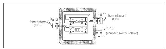
The Pg 12 cable glands on the connecting box are assigned to the initiators on delivery. The Pg 16 cable gland connects the isolating switch amplifier
