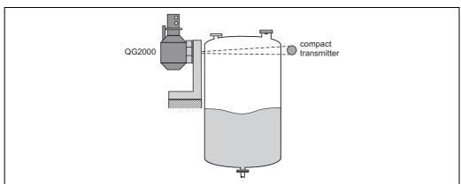
Mount the compact transmitter in a horizontal position to detect the level limit. Also mount the QG2000 so that the radiation runs horizontally.
