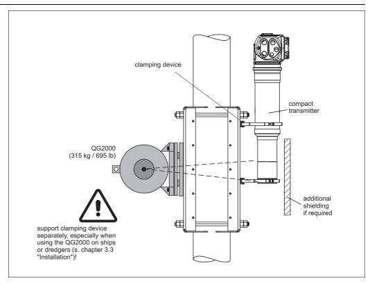
For density measurements, a clamp connection is available for pipe mounting.
