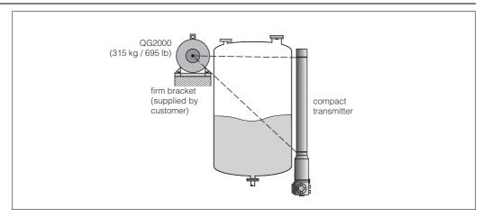
In order to ensure stable measurement and lasting radiation protection, the QG2000 must be tightly screwed onto a rugged, low-vibration bracket that can withstand a weight of 315 kg (695 lb) under all operating conditions. Additional supports are generally required when mounting directly onto the vessel. A fastening for a crane on the QG2000 is provided for transporting it.
