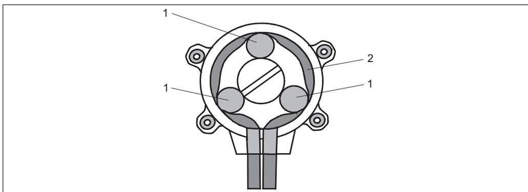
Fig. 16: Routing of pump tubing through rollers
