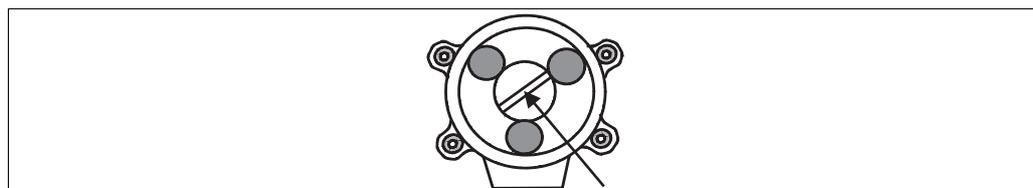
Fig. 15: Check slot for pump rotation
