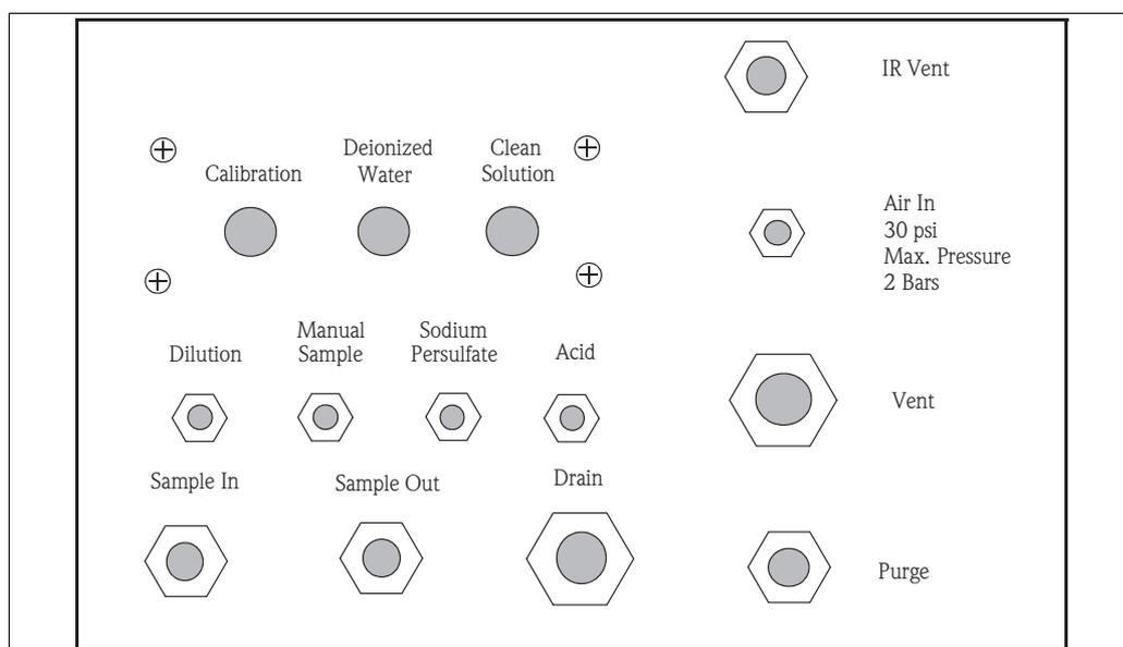
Fig. 6: Connection panel for gas and liquid connections
