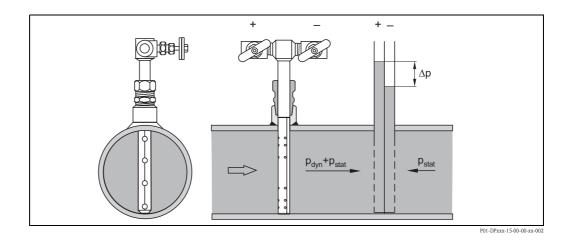
The front of the Pitot tube is exposed to the static pressure  $p_{stat}$  plus the dynamic pressure  $p_{dyn}$ . The side and the back of the tube is exposed only to the static pressure  $p_{stat}$ . The resulting **differential pressure**  $\Delta p$  can be used to calculate the **flow rate**  $\Omega$ .
