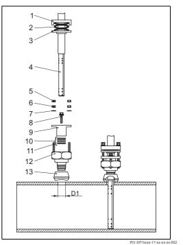
1: Load plate 2: Load springs 3: Indicator ring 4: Sensor 5: Jam nuts 6: Load nuts 7: Lock washers 8: Packing bolts 9: Follower 10: Packing rings 11: Studs 12: Spring lock body 13: Welding socket
