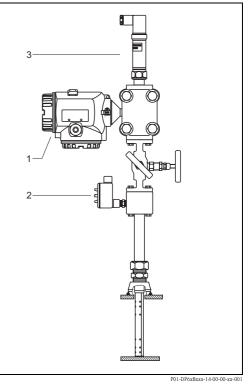
1: Deltabar S differential pressure transmitter
