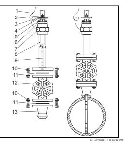
Safety cable 2: Jam nut 3: Retaining nut
