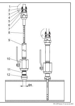
Safety cable 2: Jam nuts 3: Retaining nuts
