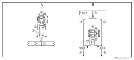
A: Preferred configuration B: Alternative configuration (if the transmitter cannot be mounted above the pipe) 1: Pitot tube 2: Shut-off valves 3: Three-valve manifold 4: Deltabar differential pressure transmitter 5: Separator 6: Drain valve
