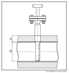
*ID:* Inner pipe diameter *H:* Thickness of the insulating layer
