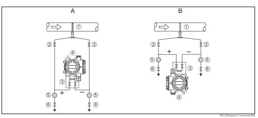
A: Preferred configuration B: Alternative configuration (requires less space; only possible for clean media) 1: Pitot tube 2: Shut-off valves 3: Three-valve manifold 4: Deltabar differential pressure transmitter 5: Separator 6: Drain valves
