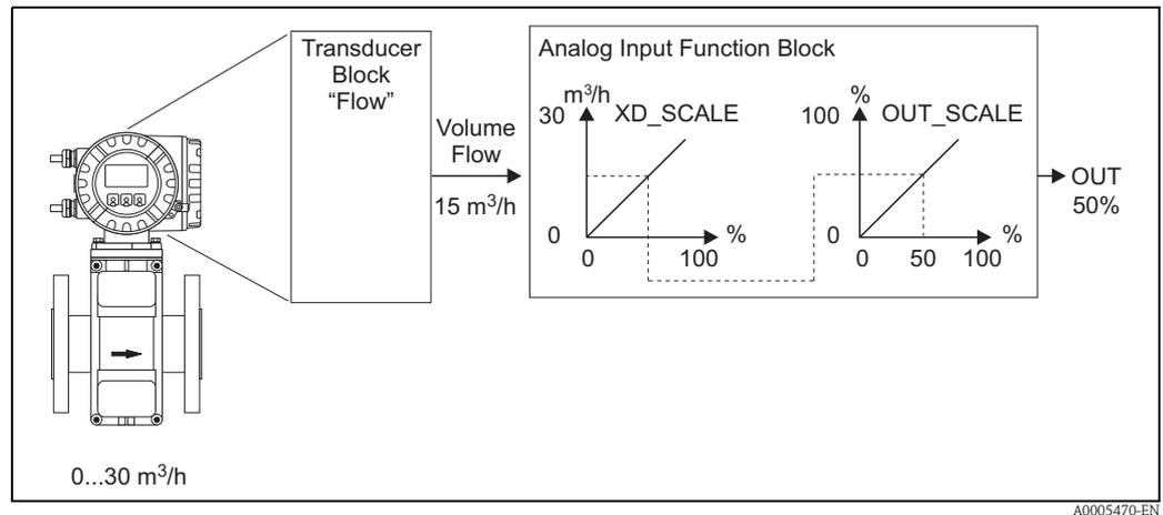
Abb. 4: Example for rescaling the input value
