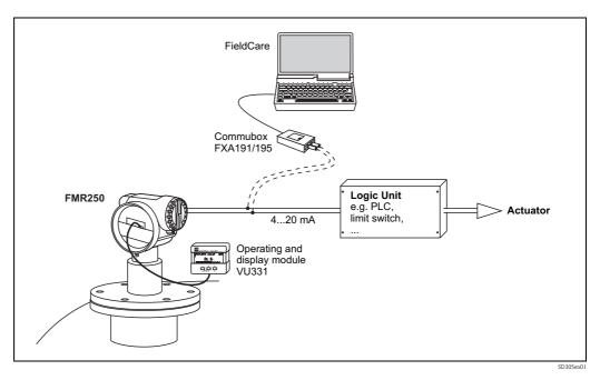
An analog signal (4 to 20 mA) in proportion to the level is generated in the transmitter. This is sent to a downstream logic unit (e.g. PLC, limit signal transmitter, etc.) where it is monitored to determine whether it is above a specified limit value.
