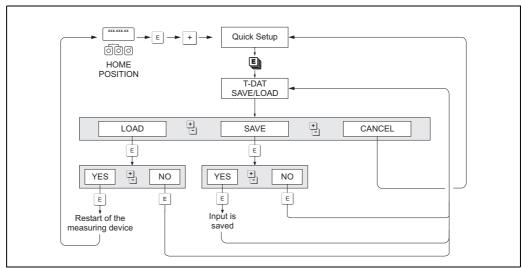
Data backup/transmission with T-DAT SAVE/LOAD function
