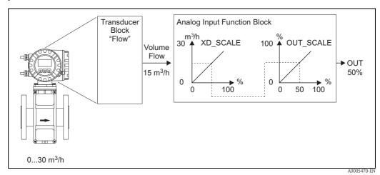
Fig. 4: Example for rescaling the input value
