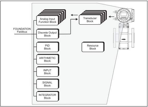
Fig. 1: Promag 53 FOUNDATION Fieldbus blocks
