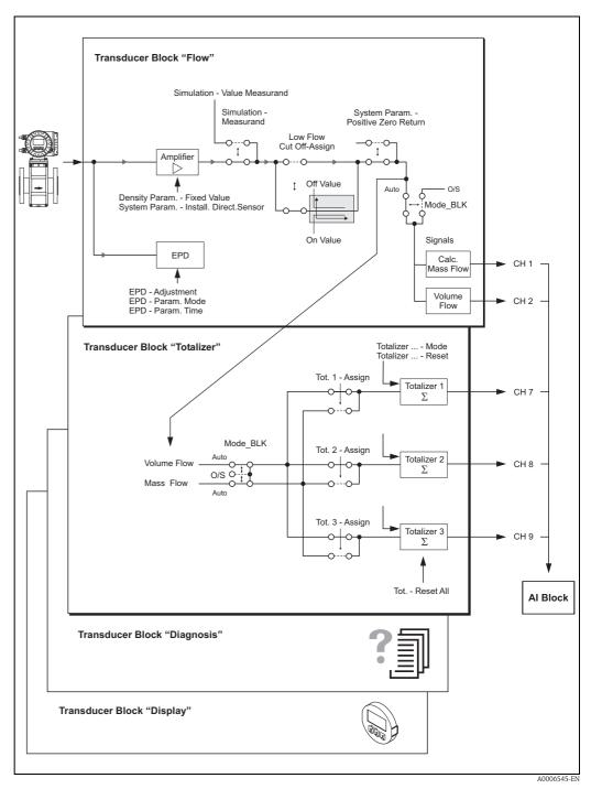
Fig. 2: Internal structure of the individual Transducer Blocks
