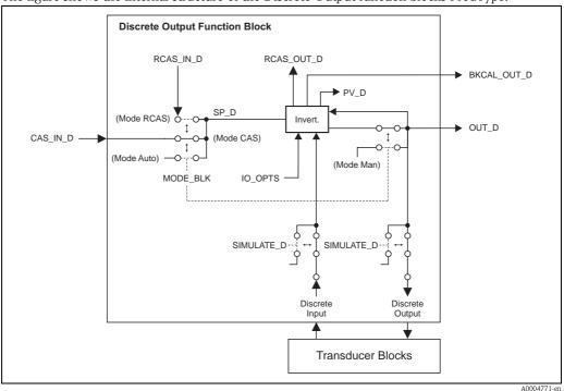
Fig. 5: Signal processing in the Discrete Output function block
