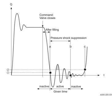
$\textcircled{1} = on \ value \ (low \ flow \ cut \ off), \ \textcircled{2} = off \ value \ (low \ flow \ cut \ off)$
