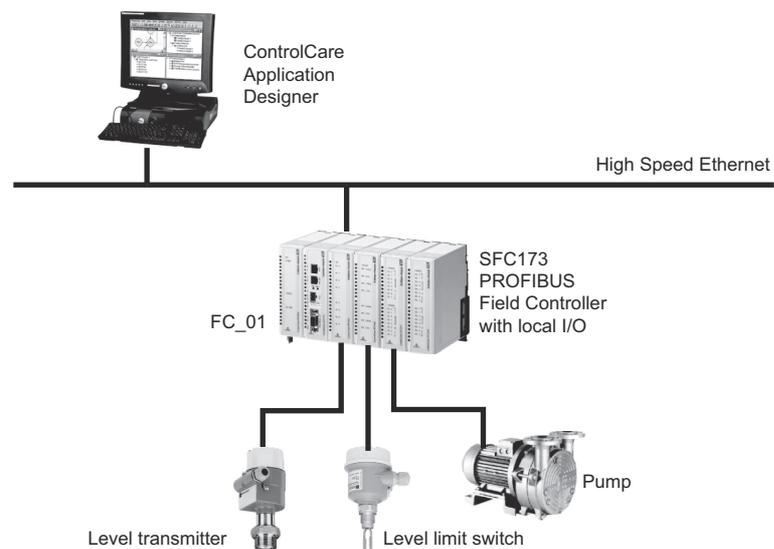
Fig. 2-4 Network for application example
