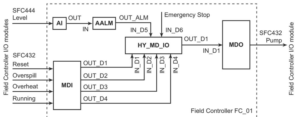
Fig. 2-3 Control strategy for pump control application
