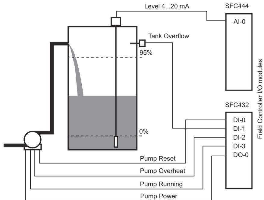
Fig. 2-1: Overview of pump control for tank filling
