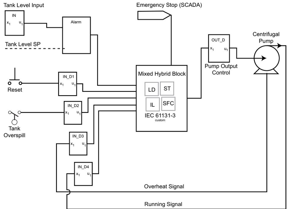
Fig. 2-2: Schematic diagram of pump control application
