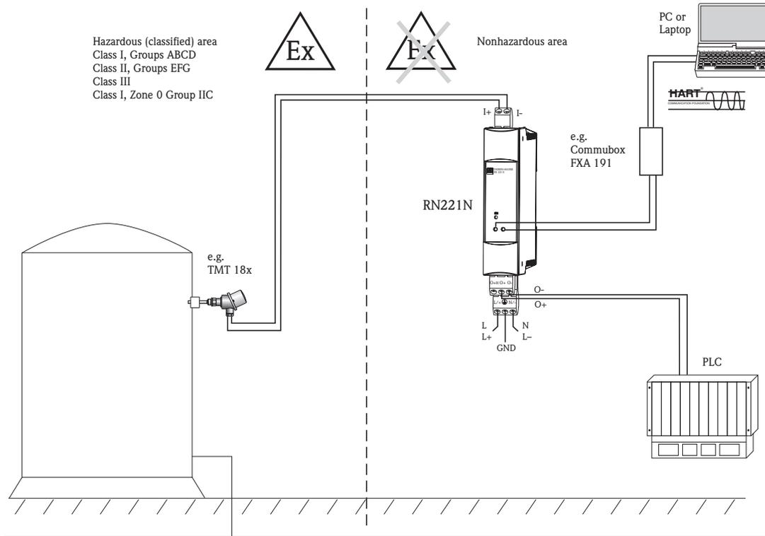
Typically the RN221N is mounted in the non-hazardous area and the split between the supply voltage and the intrinsically safe voltage occurs in the device itself. The cables powered by the RN are then fed into the hazardous area where they power the two wire transmitter. The RN221N transmits the measured signal received from the hazardous area to the non-hazardous area equipment. HART signals are bi-directionally transmitted.
