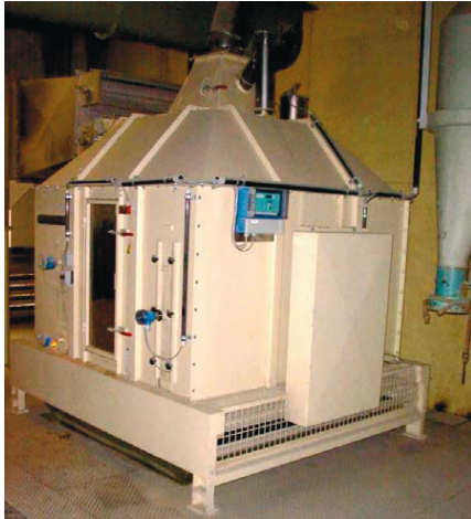
Soliphant T point level detection in pellet cooler
