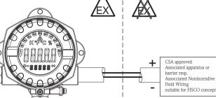
RID14 with electronic insert for Profibus PA/Foundation Fieldbus Concept FISCO Ui (Vmax) 17.5 V 24 V 500mA 250mA Ii (Ìmax) 5.5 W 1.2 W Pi (Pmax) Ci < 5nF Li < 10 tiH Leakage current ≤ 50 µA
