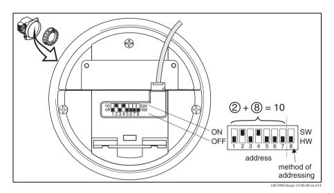
Hardware addressing comes into operation, when DIP switch 8 is in the position "HW (OFF)". In this case the address is determined by the position of DIP-switches 1 to 7 according to the following table:
