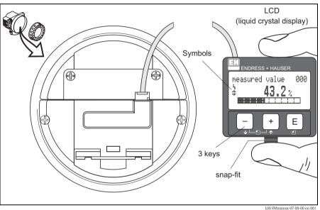
The VU331 LCD display can be removed to ease operation by simply pressing the snap-fit (see graphic above). It is connected to the device by means of a 500 mm cable.
