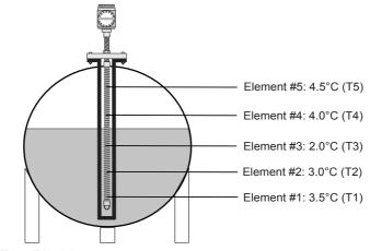
Formula:(T1 + T2 + T3) / # of element in liquid phase = Average temperature  $(3.5^{\circ}C + 3.0^{\circ}C + 2.0^{\circ}C) / 3 = 2.83^{\circ}C$
