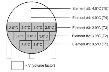
$(3.5^{\circ}C \times 2 + 3.0^{\circ}C \times 3 + 2.0^{\circ}C \times 4) / (2 + 3 + 4) = 2.67^{\circ}C$
