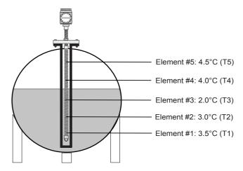
Formula:(T1 + T2 + T3) / # of element in liquid phase = Average temperature $(3.5^{\circ}C + 3.0^{\circ}C + 2.0^{\circ}C) / 3 = 2.83^{\circ}C$
