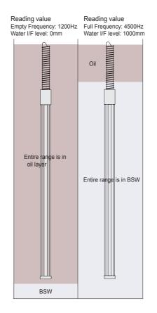
(4500Hz -1200Hz) / 1000mm = 3.3Hz / 1mm
