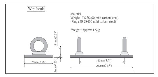
Actual tensioning can be completed with SUS316 stranded 3mm diameter tension wire between wire hook and top anchor.
