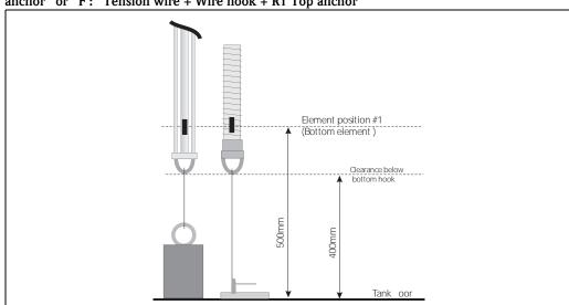
Mounting attachment B: "High profile anchor, D120", D: "Tension wire + Wire hook +NPT1 Top anchor" or "F: "Tension wire + Wire hook + R1 Top anchor"
