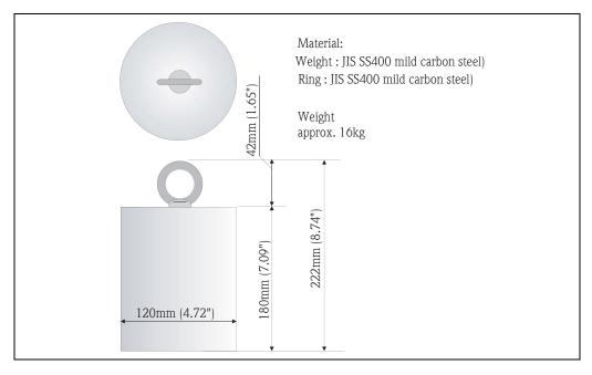
Different dimensions, weight and material for the anchor weight are also available.
