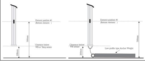
"Low profile anchor weight" is provided to anchor WB probe and to measure accurately water bottom range. When installing NMT539 on small tank nozzle [max.50A (2")] in operating tank, it is available as mounting attachment for converter + temperature probe version. Both the temperature probe and WB sensor with "Low profile anchor weight" at 100: Mounting attachment option (see Ordering Information) should have 200 mm (8") of bottom clearance from the edge of probes.
