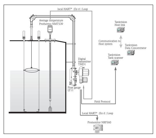
Average temperature data is transmitted to transmitter TMD1 via local HART  $^{\!\scriptscriptstyle \odot}$  communication.
