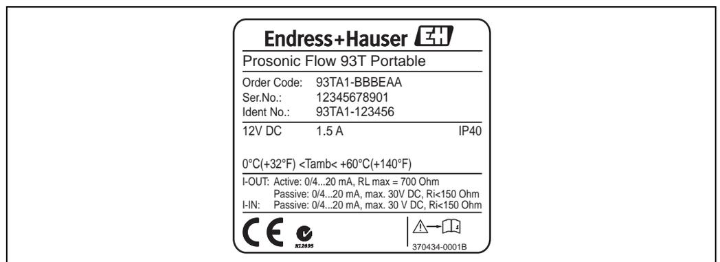
Fig. 1: Nameplate specifications for the "Prosonic Flow 93T" transmitter (example)
