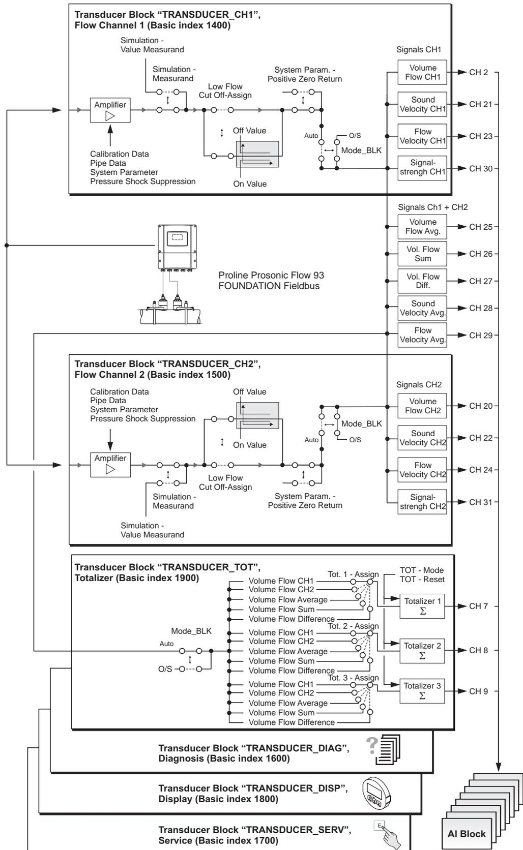
Fig. 2: Internal structure of the individual Transducer Blocks
