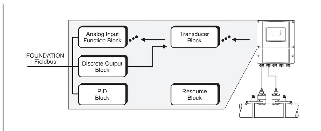
Fig. 1: Prosonic Flow 93 FOUNDATION Fieldbus block model
