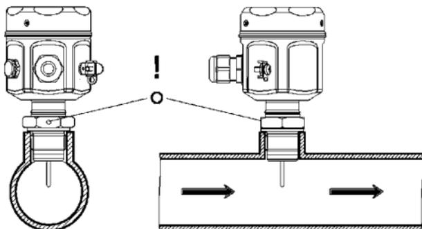
If the sensor is not installed as above it may affect the performance of the instrument.
