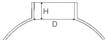
Guidelines provided relate to the dimensions of the mounting boss and not the process pipe!
