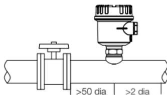
Directly after pumps, fans and compressors.
