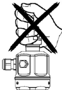
Place sensor end up. Sensor impact may cause damage.
