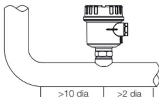
Directly downstream of isolation and control valves especially if partially opened.
