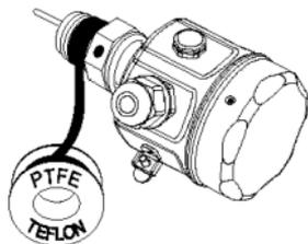
Always use a spanner to tighten the t-trend process connection.
