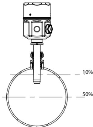
For pipe diameters  $\geq DN250$
